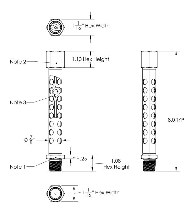
1) Process Fitting is 1/2" NPT Male 2) Instrument Fitting is 1/2" NPT
